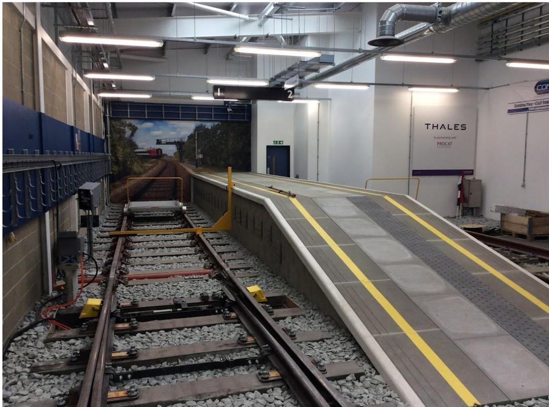
The equipment provided by Thales was match funded by the Skills Funding Agency (SFA) and these funds were used to build the network infrastructure around the telecommunication systems, along with additional elements such as cabling, the track and the station.
